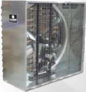
36" Belt drive exhaust fan in box housing, 6-wing blade,
